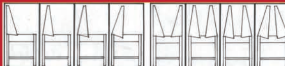
ILLUSTRATION ABOVE SHOWS HOW WE1 & WE2 SHIELDS TILT (4 POSITION) TO CONTROL HEAT DIRECTION
